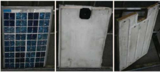
Figure 1. Broken glass of the polyethylene slab prototype and heat exchanger at its back (left and middle). Epoxy resin heat exchanger (right).
