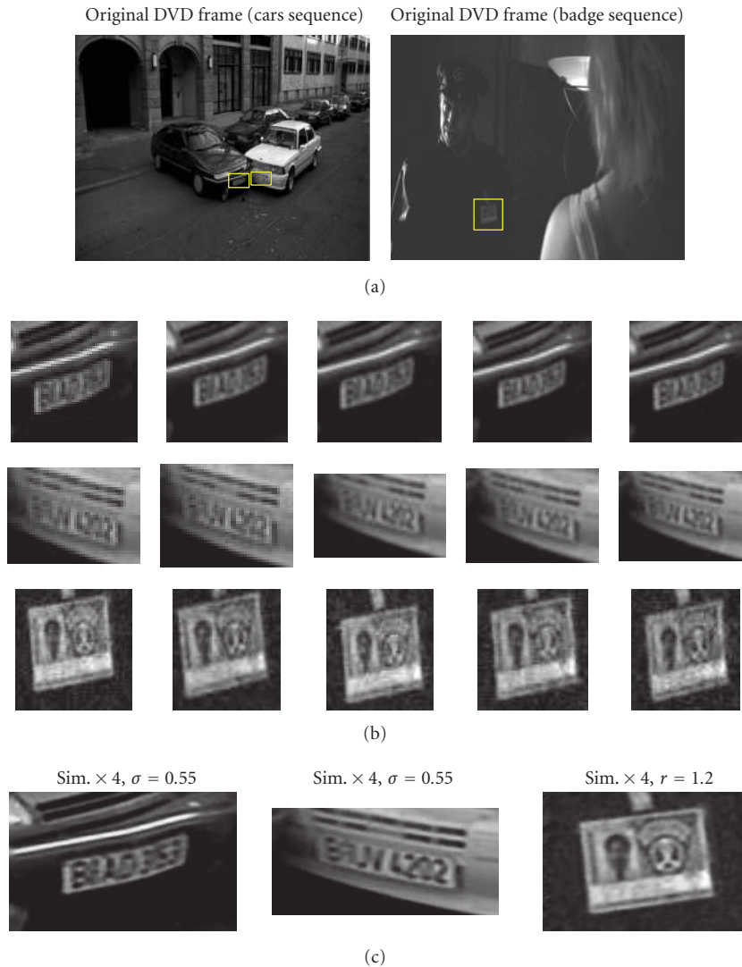
FIGURE 8: Results from the simultaneous super-resolution, image registration, and prior parameter updating scheme applied to the movie Lola Rennt on DVD. (a): two raw DVD frames. (b): five low-res frames from each sequence (black car's number plate, white car's number plate, security guard's ID badge). (c): the same image regions super resolved using the simultaneous method. In the case of the security guard's ID badge, intensities have been scaled for ease of viewing. Please refer to the text for notes on the aspect ratios involved when working with DVD frames.
