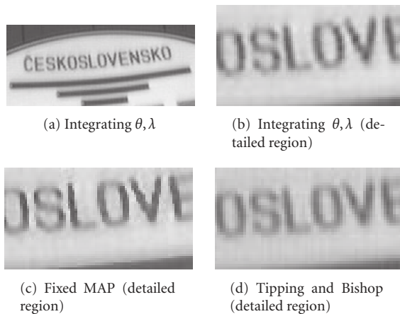
FIGURE 11: (a) The full super-resolution output from our algorithm. (b) Detailed region of the central letters, again with our algorithm. (c) Detailed region of the regular Huber MAP super-resolution image, using parameter values suggested in [18], which are also found to be subjectively good choices. The edges are slightly artificially crisp, but the large smooth regions are well regularized. (d) Close-up of letter detail for comparison with Tipping and Bishop's method of marginalization. The Gaussian form of their prior leads to a more blurred output, or one that over fits to the image noise present on the input data.
