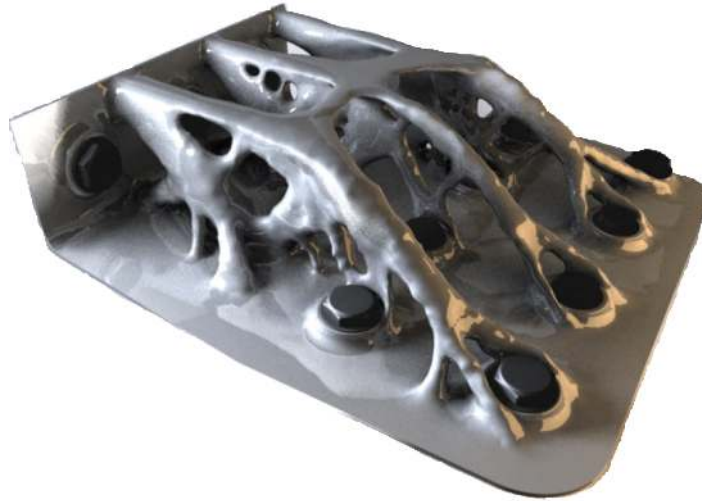
Figure 1.1: Example of a complex shaped part that is effortlessly produced with selective laser melting (SLM). The part is a topology optimised aerospace bracket and shows the match between topology optimisation and additive manufacturing. [8].
