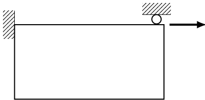
Figure 9.3: Schematic drawing of the tension beam problem indicating the design domain, support and applied force.
