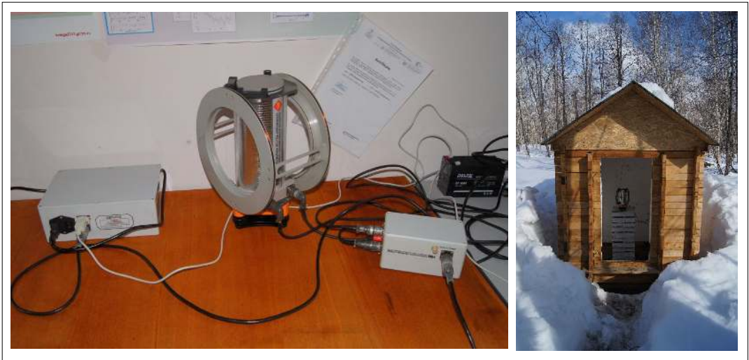
Figure 1. Vector magnetometer POS-4. Left panel: a UPS is to the left, sensor (solenoid and ring system on the carrier) is in the center, electronic unit is to the right. Right panel: POS-4 hut, magnetometer sensor is mounted on a pillar made of building glass stones, the removable hut door is on brass bolts (March 2016)
