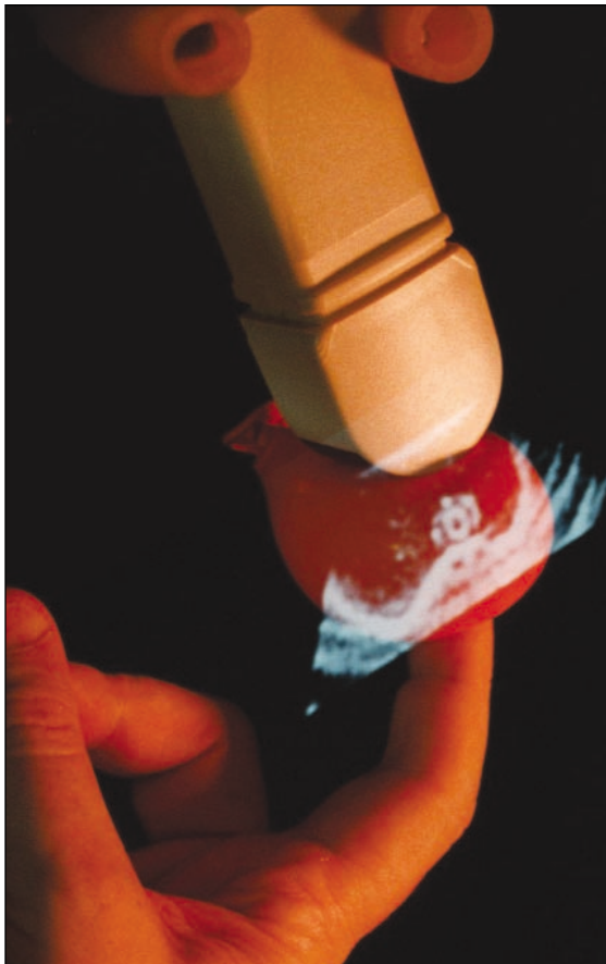
Figure 6. Scan of a fluid-filled balloon containing a short piece of rubber tubing (tubing is seen in cross section). The operator's finger is seen pressing into the balloon against the tubing.
