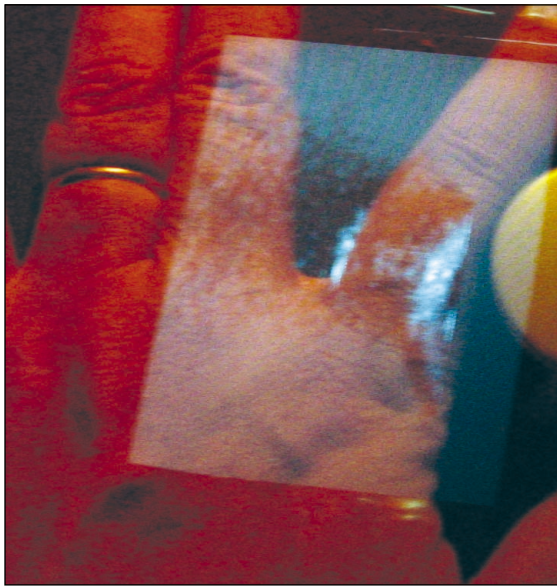
Figure 5. Scan of a finger using the portable version of the device, as seen through the half-silvered mirror.
