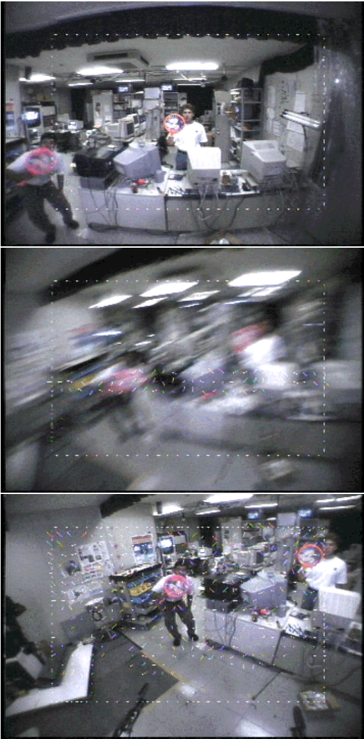
Figure 4: Snap shots of the robot's peripheral view before, during, and after an attentional head-eye saccade, taken at 30 Hz sampling rate. Superimposed on the images is the visual flow field.
