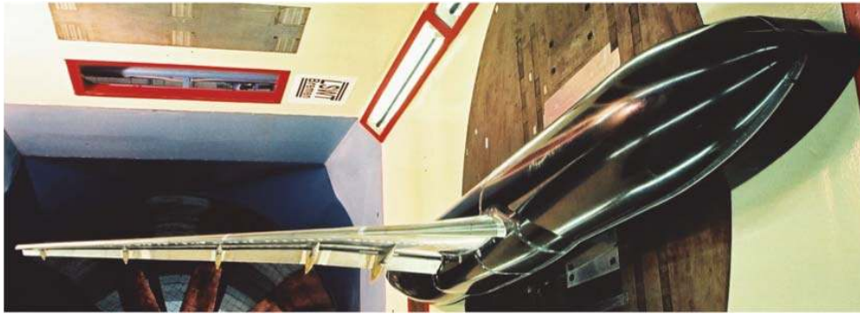
Figure 1. Photograph of DLR-F11 high lift model in the B-LWST wind tunnel.
