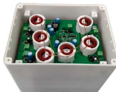
Fig. 10. Solar inverter cell using 10 kV SiC MOSFET.
