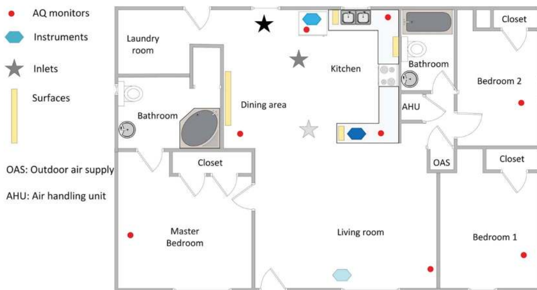
Fig. 1 The UTest house floor plan includes a large open living room and kitchen space, including a sink and stove. The markers indicate instrument/inlet general locations. The bathroom doors were sealed with the master bathroom's exhaust fan left on; all other interior room doors were kept open. Three sets of large instruments were maintained inside the house (light blue hexagon in living room: \text{HO}_x , HONO and spectral radiometer measurements; medium blue hexagon in kitchen: \text{NH}_3 measurement; dark blue hexagon between kitchen and living room: aerosol and biological aerosol size distribution measurements). Low-cost air quality monitors were placed on top of the cupboards separating the kitchen from the living room area, and in the living room and bedrooms (red circles). Multiple vertical sampling surfaces were placed in the dining area and kitchen (yellow bars). Inlets for external sampling were located in the kitchen area (stars; black: SVTAG inlet; light grey: \text{O}_3 , \text{NO}_x , \text{SO}_2 , \text{CO}_2 and GC measurements of VOCs; medium grey: all other measurements). The locations of the outdoor air supply and air handling unit are indicated. The dishwasher is under the counter to the left of the sink, and the refrigerator between the sink and SVTAG inlet.
