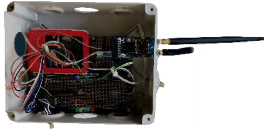
Fig. 2: Picture of a test node. Four such test nodes are used in the experiments, each equipped with an AT86RF215 radio communicating on both 2.4 GHz IEEE802.15.4 O-QPSK and sub-GHz IEEE802.15.4g OFDM.
