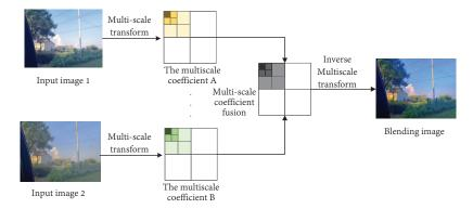
Figure 10. Image integration method based on multi-scale [2].
