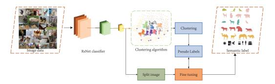
**Figure 30.** An unsupervised semantic algorithm. The framework uses a RetNet classifier for classification and then uses a clustering algorithm to cluster features. Finally, similar features are clustered into the same set of semantic labels, and the semantic labels of the groups are obtained by fine-tuning. Reproduced with permission of [289], Copyright of 2023 IEEE Transactions on Pattern Analysis and Machine Intelligence.
