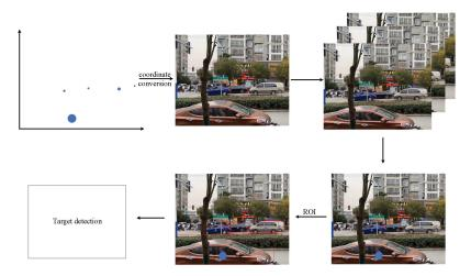
Figure 11. Data-level-based image and radar data fusion [2].
