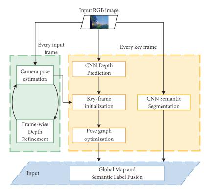
Figure 28. The CNN–SLAM structure [270].
