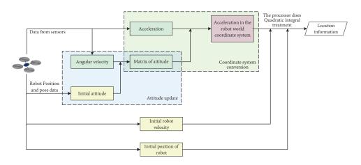
Figure 22. Robot pose determination process.
