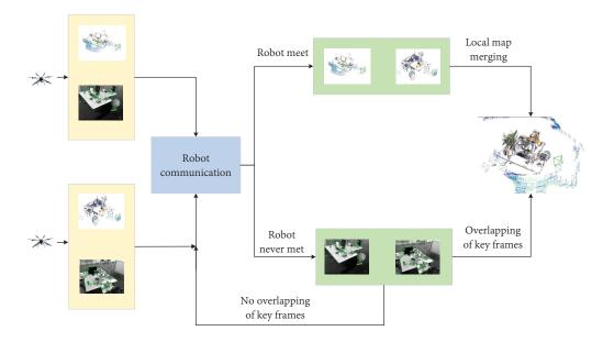
**Figure 24.** Block diagram for determination of overlapping areas. An office map is taken as an example, where two robots build a map around a desk, communicate with each other after forming their mapping, and locally fuse the locations where the keyframes overlap when they meet. The keyframes are detected when the robots do not meet, and map fusion is performed when the keyframes overlap. When the keyframes do not overlap, the mapped data are used to communicate with the robots again.
