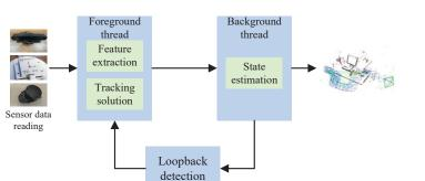
Figure 14. Schematic diagram of the SLAM framework.
