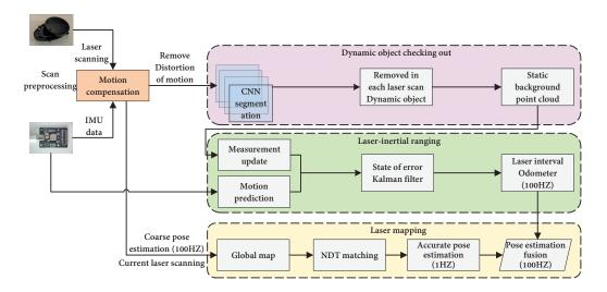
**Figure 19.** A loosely coupled LIO-SLAM model [90]. The system is composed of four sequential modules, including a laser inertial ranging module and a laser mapping module. Through the cooperation of the four modules, robust motion estimation and motion mapping in highway environments can be realized.
