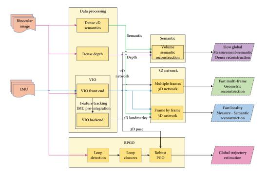
the earlier version, its robustness and accuracy were greatly improved. Figure 29 shows the workflow of supervised learning multi-robot semantic SLAM.
