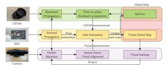
Figure 20. A kind of VIL-SLAM system structure diagram [198].
