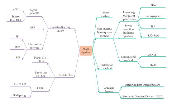
**Figure 16.** Summary of SLAM algorithms. Single-sensor SLAM methods were divided into two categories—according to traditional filtering methods and modern optimization algorithms—and the known SLAM algorithms with high frequency were classified. In this way, the structural diagram of the SLAM algorithms was obtained.
