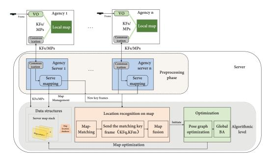
**Figure 25.** Centralized architecture schematic diagram. The agent robot runs a real-time VO and maintains a local map of size N in its memory, as well as a communication module to exchange data (keyframes with map points and reference frames of the current position) with the server. Servers are ground stations that perform non-time-critical and computationally expensive processes.
