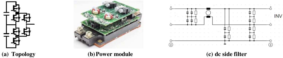
Figure 12. GE silicon carbide 1-MW inverter.
