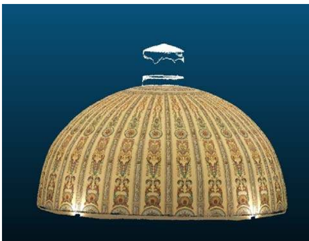
Figure 11: TLS point cloud
