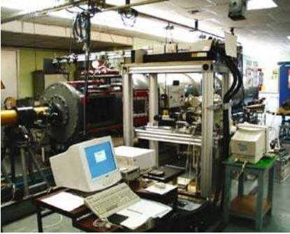
Fig. 11. ISL shock tunnel with PIV system ( Haertig et al. 2002 )
