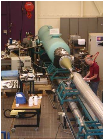
Fig. 10. Hypersonic Test Facility Delft (HTFD) with installed PIV system
