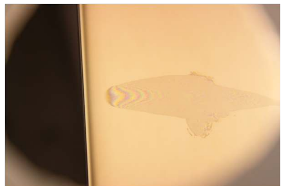
Figure 25. Fringe on test nickel plated wing, using 10cSt oil and compressed air to create fringe. Wing is lit with a diffuse reflector and mercury vapor bulbs. The color bands on the fringe appear because no dichroic filter was used.
