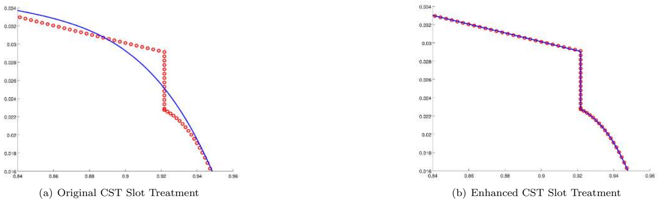
Figure 10. This compares the original CST treatment of the slot associated with CCA. Notice that CST’s smoothing characteristic completely removes the slot while the enhanced treatment captures it.
