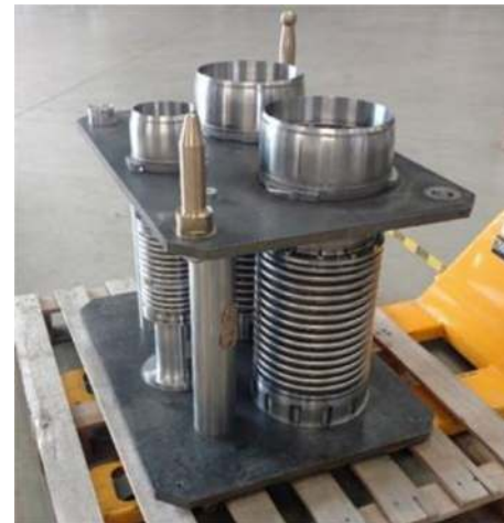
Figure 13. Pipe alignment proof-of-principle pipe module side test assembly.
