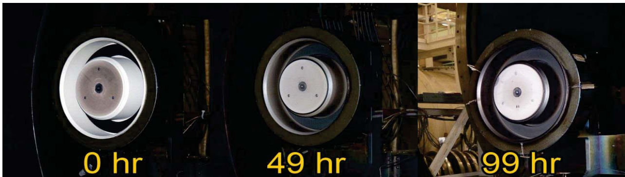
Figure 2. Photographs of the 300MS thruster inside NASA Glenn's VF5 prior to test initiation (left), after 49 hours (middle), and after 99 hours (right).
