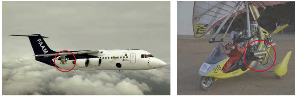
Figure 4. (left) FAAM BAe146 aircraft. The aerosol and cloud physics probes are visible mounted on the wing pylon as highlighted by the red circle. (right) ULA with the LAUVA lidar in horizontal pointing mode highlighted by the red circle.
