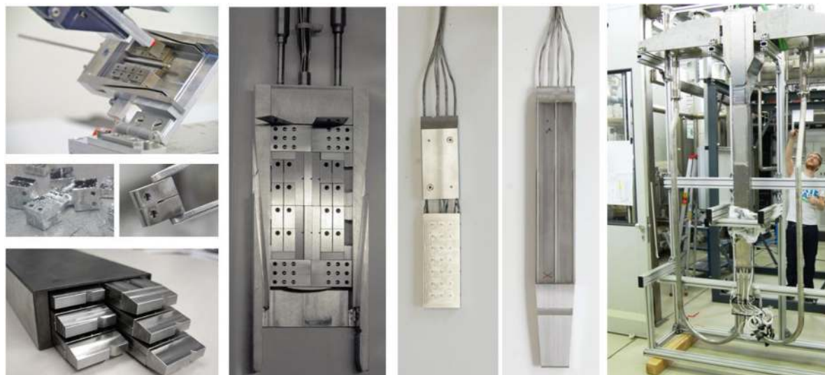
Figure 18. Top left: small specimens during assembly and recovery (NaK coating visible). Bottom left: rigs inserted in the HFTM body. Middle: complete specimen set, capsule, and completely assembled rig. Right: HFTM-DC prototype during integration into the HELOKA-LP helium loop.
