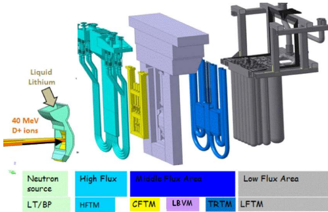
Figure 9. Target and TMs arrangement in the TC—the neutron cloud and the TMs are shown symbolically.
