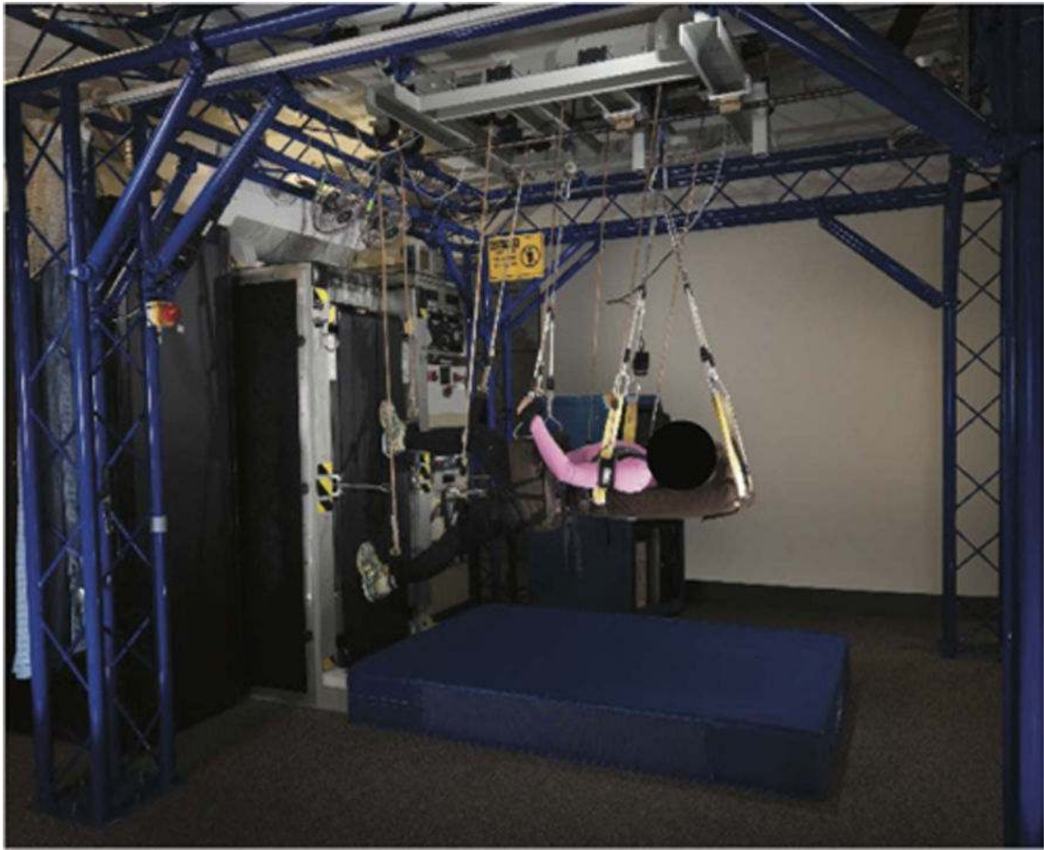
FIGURE 2. Specialized vertical treadmill used for interval aerobic training for exercising participants. Subjects were supported by a harness and maintained in a supine, horizontal position during exercise.
