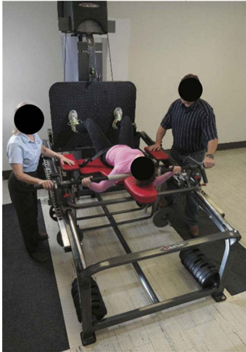
FIGURE 3. Horizontal squat device used for resistance exercise training. This NASA custom-built device enabled performance of a squat weightlifting exercise while maintaining a horizontal position.
