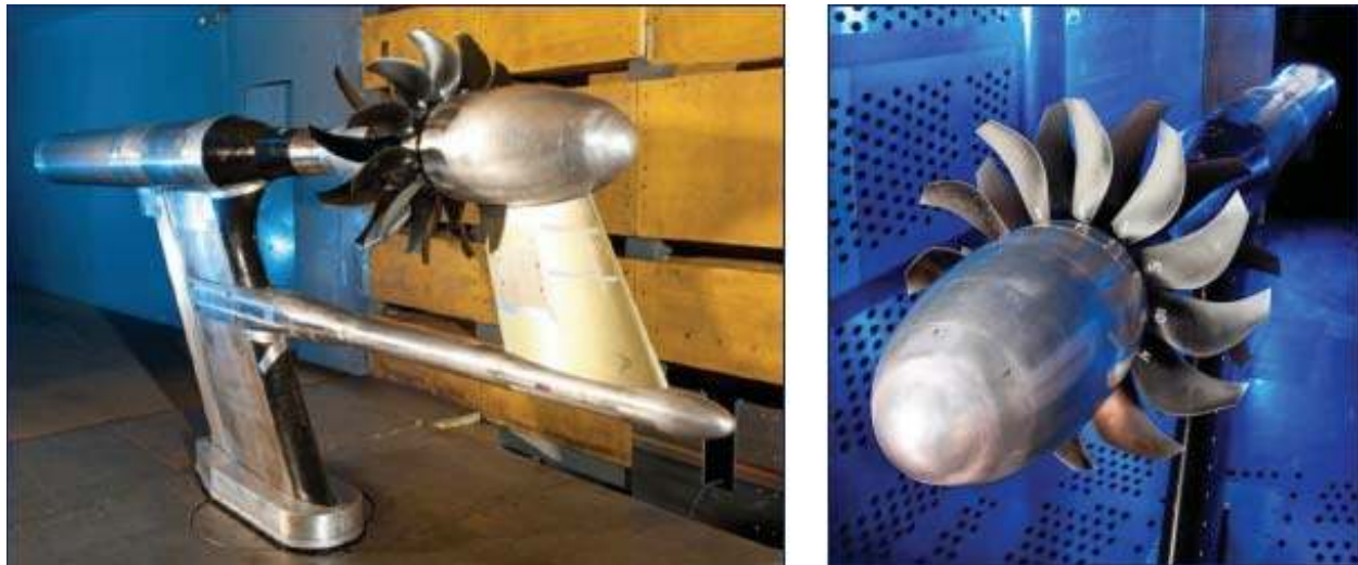
Figure 8: The Open Rotor Propulsion Rig installed in the 9x15 Low Speed wind tunnel on the left and on the right it is installed in the 8x6 Transonic Wind Tunnel in preparation for performance testing at cruise Mach of ~0.8.
