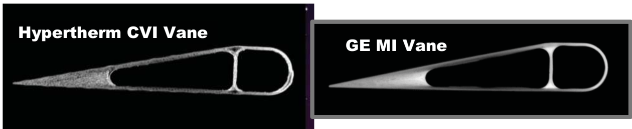
Figure 20: CT images of the Hypertherm CVI & the GE MI vanes. Note the delamination in the Hypertherm vane.
