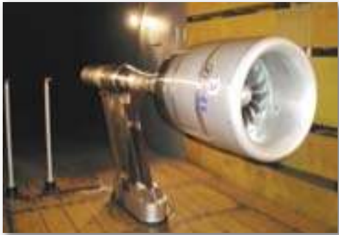
Figure 12: (a) P&W Geared TurboFan installed in the 9x15 low speed wind tunnel. (b) Over-the-Rotor and Soft Vane noise reduction technologies.
