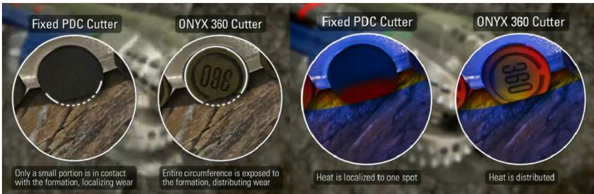
Fig. 19 The comparison of fixed PDC cutter and ONYX 360 cutter
