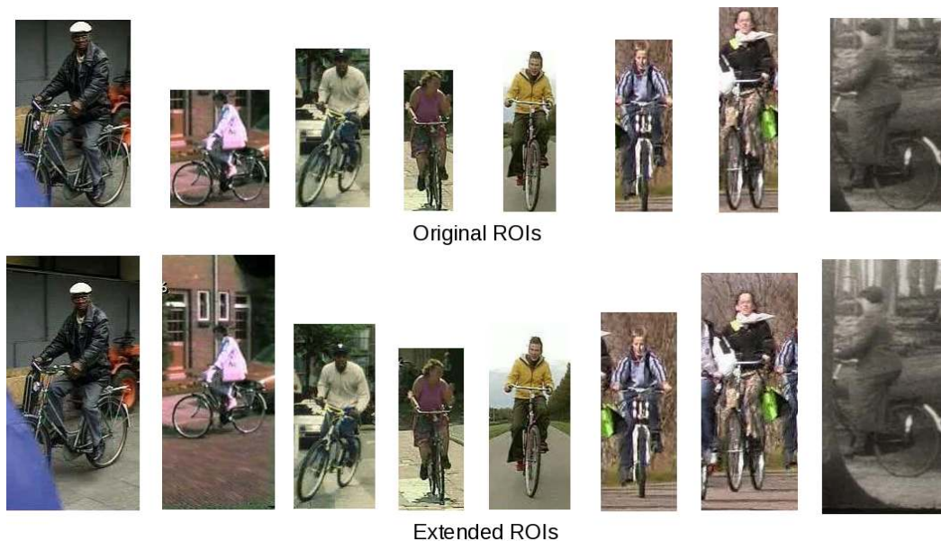
Figure 2: Top row shows the examples of original ROIs for class Person-riding-a-bicycle, and their extended ROIs are shown in the bottom row. Note that all the extended ROIs have same aspect ratio.
