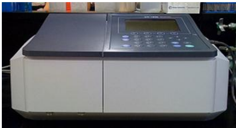
Fig. 3.2: A UV-Spectrophotometer (UV-1800, Shimadzu) for measuring concentrations of potassium permanganate.
