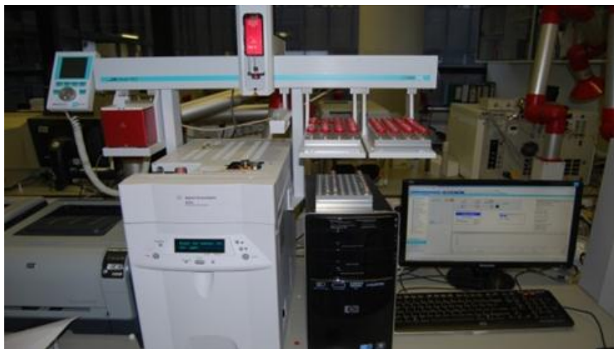
Fig. 3.1: Gas chromatograph (Agilent 6850) for measuring concentrations of the target compounds.
