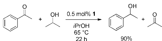
Scheme 7. Catalytic transfer hydrogenation of acetophenone in isopropanol. For further details see Table S2 and Figures S35–37.
