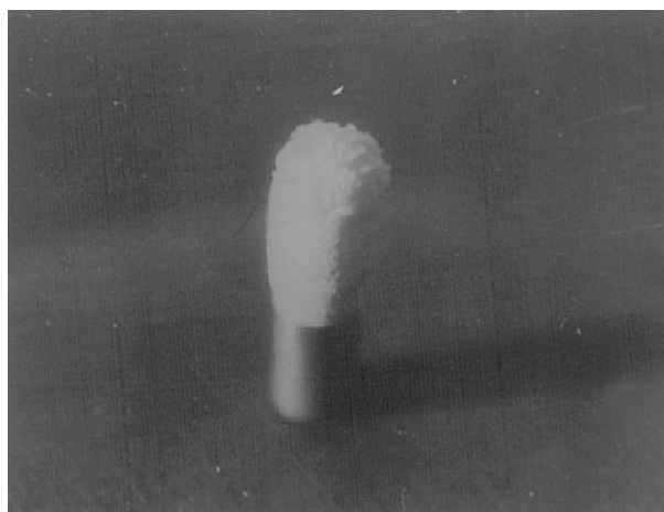
Figure 4. Mass left after oxidation of a Y–Si–Al–O–N glass (Das 1993).
