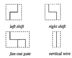
Each figure is simply a "wiring" diagram, and when two figures are placed with their wires touching, a value is transmitted through each wire in the natural way. Values can only be transmitted down in the vertical direction, though they may be transmitted either left or right horizontally.
