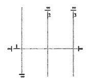
There is no explicit gadget corresponding to a vertical wire. A value is transmitted vertically as the extension of a line segment within some gate. The gadgets for the  $\vee$  gate and inverter, respectively, are:
