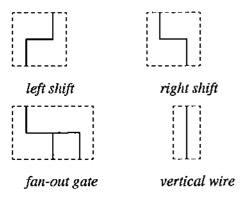
Each figure is simply a "wiring" diagram, and when two figures are placed with their wires touching, a value is transmitted through each wire in the natural way. Values can only be transmitted down in the vertical direction, though they may be transmitted either left or right horizontally.
