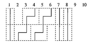
The first and third phases consist of the same operation: routing wires without crossing or branching. The second phase is an even simpler process of copying values into adjacent columns to the right. We describe its operation first.
