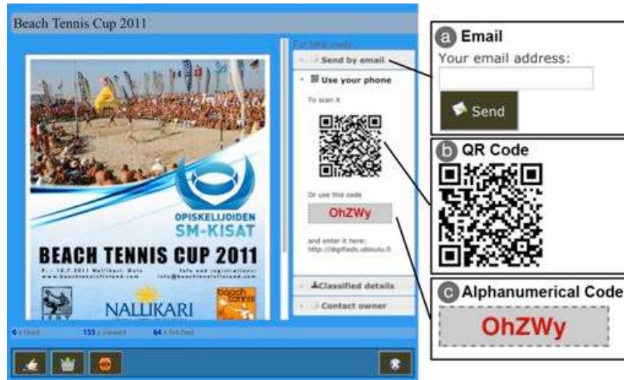
Fig. 11. Exchanging Content: Users can send digifieds to their a) email address or transfer them to their mobile phone using either the b) QR code, or the c) alphanumeric code.
