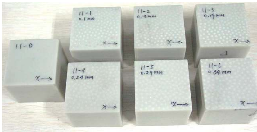
Figure 8. Synthetic rock samples containing penny-shaped fractures. The sample 11–0 is the reference sample with no fractures, whereas samples 11–1 to 11–6 have the same fracture density and radius, but with the increasing fracture thickness, as indicated in the figure (0.1 – 0.34 mm).
