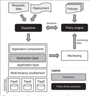
**Figure 1 Concept diagram.** High-level overview of the policy-driven mechanism of the proposed PaaSHopper middleware.
