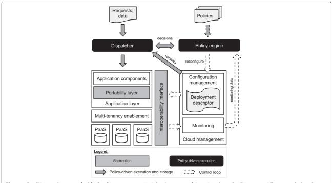
**Figure 5 PaaSHopper integrated with cloud management.** High-level overview of the policy-driven PaaSHopper middleware, including the integration with cloud management services such as monitoring and configuration management.
