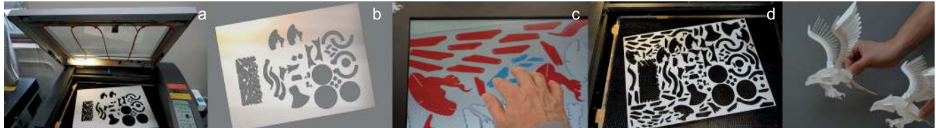
Figure 1. PacCAM supports users in packing 2D parts by capturing materials in a CNC machine (a) and using the captured materials (b) in a dedicated user interface based on 2D rigid body simulation and snapping (c), resulting in optimized utilization of material for efficient fabrication (d).
