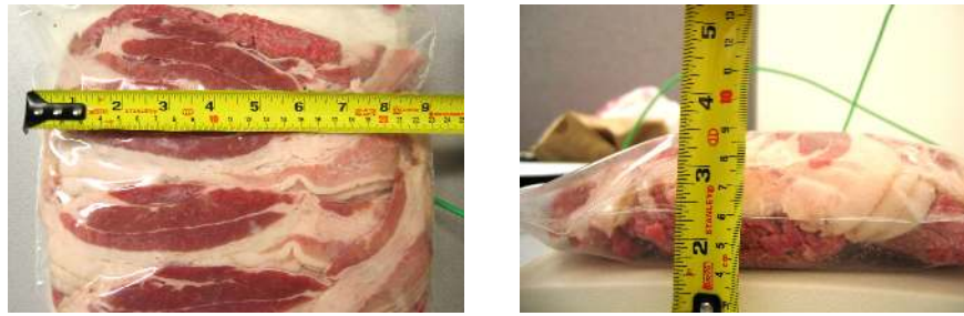
Fig. 8. To simulate implantation in a human, we placed the WISP in a bag containing bacon and ground beef.
