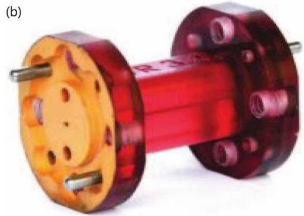
Fig. 18. Photographs of metal-coated WR3.4 WGs printed with the SLA-based printer. Figures from [144].
