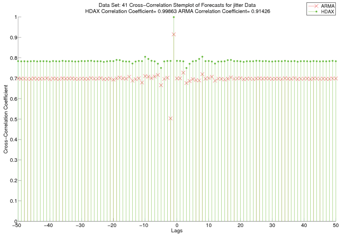
Figure 4.21: Stemplots of cross-correlation of HDAX forecasts and target jitter time-series for dataset 41 together with those of ARMA
