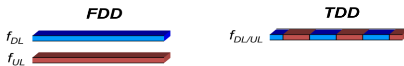
Figure 2-8: FDD & TDD in LTE
