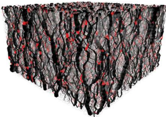
FIG. 18. (Color online) Snapshot of radial forces for the sample S5. Line thickness is proportional to the radial force. Mobilized forces ( I_c \simeq 1 ) are in red.
