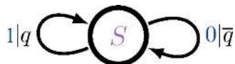
Figure 3 Hägg-machine for the IID process. When q = 1 , the IID process generates a string of 1's, which is physically the 3C^+ stacking structure. Conversely, when q = 0 , the structure corresponds to the 3C^- structure. For q = 1/2 , the MLs are stacked as randomly as possible. Here and elsewhere we adopt the convention that a bar over a variable means one minus that variable, i.e. \bar{q} \equiv 1 - q , with q \in [0, 1] .
