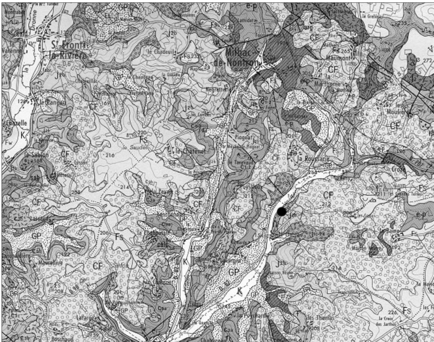
Fig. 4. Geological map of area around the Villars Cave (dot) - (C) : Cretaceous; (J) : Jurassic where the Villars Cave develops (dot); (L) : Lias; at the top right (ε) : crystalline/meta-volcanic rocks ; from BRGM, Service Géologique National, Orléans, France; Thiviers Map XIX-33 1/50000.
