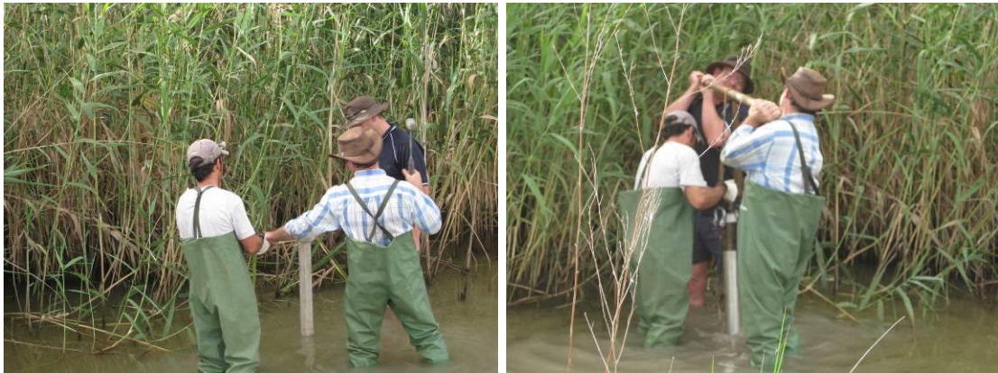
Figure 3.5. Coring at the LSW site. (Photo taken in November 2008; impaling aluminium core barrel by sledge hammer and withdrawing core barrel with strap and horizontal bar)
