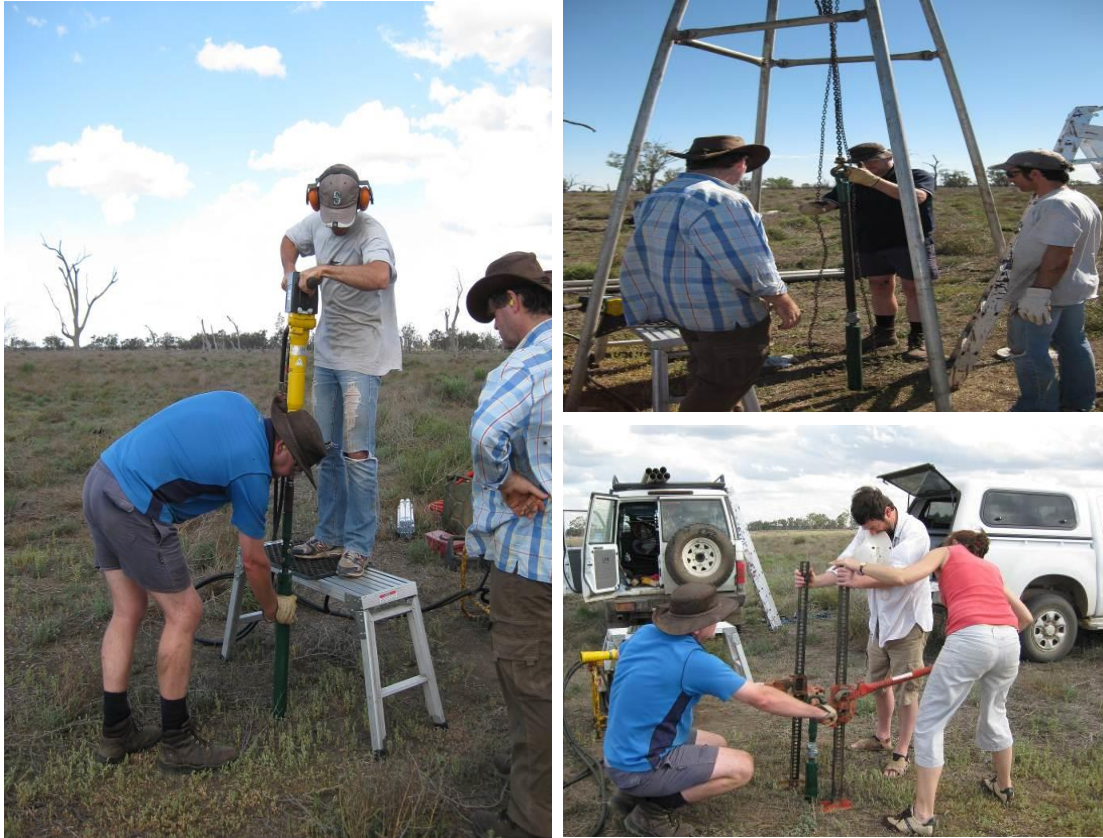
Figure 3.6. Coring at the LOLA site. (Photo taken in November 2008; Left photo - driving steel core barrel with hydraulic jack hammer; Right photos – extracting core barrel with (a) quadripod and block and tackle, (b) kangaroo jacks.)
