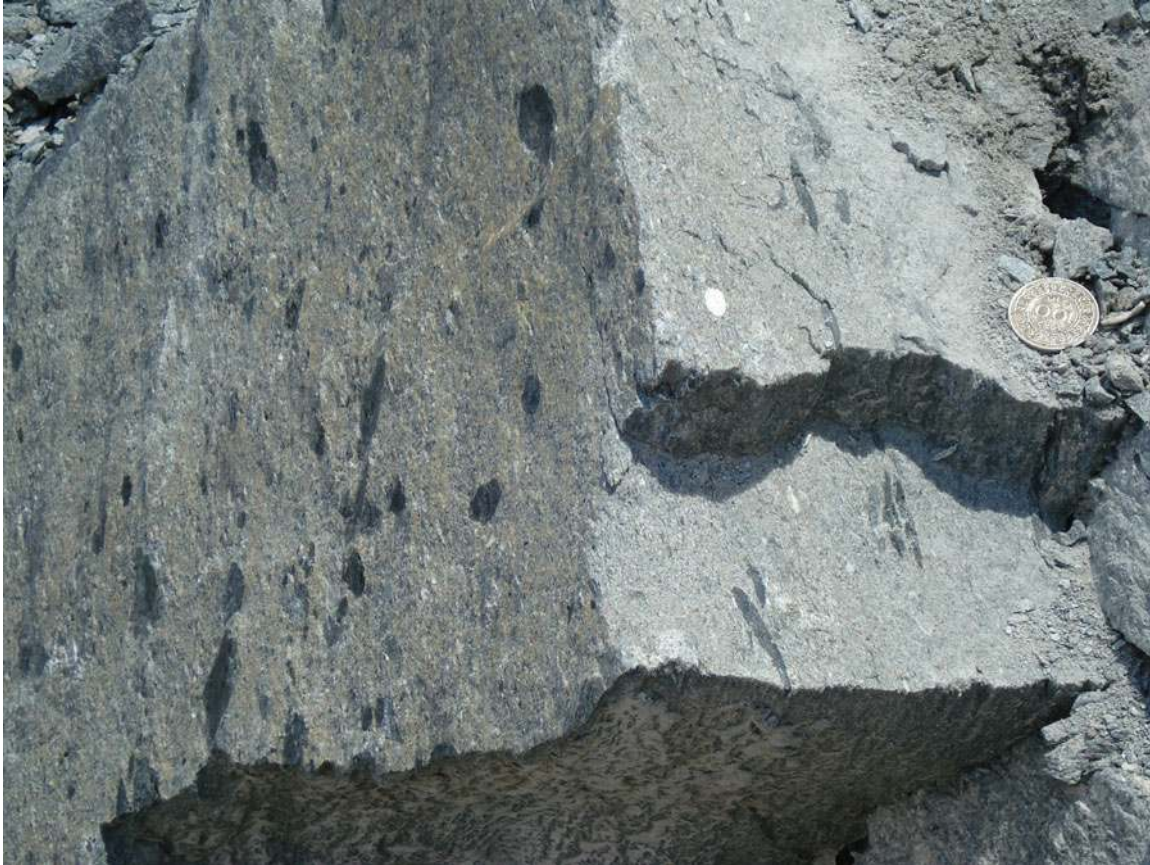
Fig. 8. Rosebel Formation meta-arenite with phyllite and quartz pebbles (left: parallel to bedding, right: perpendicular to bedding). Royal Hill pit, Rosebel Gold Mine.
