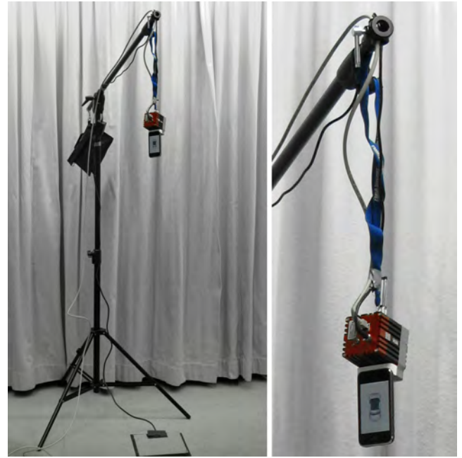
Figure 2: Hardware setup: The depth camera is mounted on top of a mobile phone in a slightly downward angle. The prototype is attached to a lanyard, such that it can be handled comfortably.
