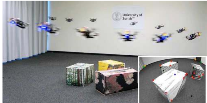
Fig. 1: An example application of our PAMPC, where a quadrotor is asked to fly at 3 m/s around a region of interest while keeping it visible in the field of view of its camera.
