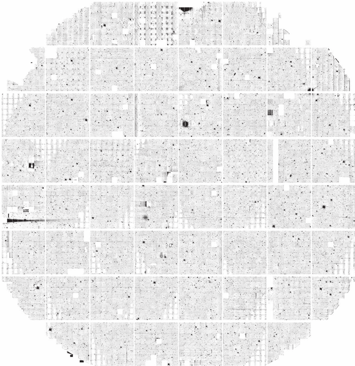
Figure 8. Glints: example of a glint on exposure o5379g0103o (2010 July 2, 45 s i_p1 filter). The source star out of the field of view creates a long reflection that extends through OTA73 and OTA63.
