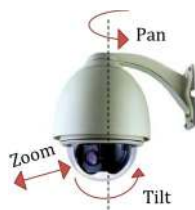
Figure 3: Mechanically steerable cameras' 3 degrees of freedom.
