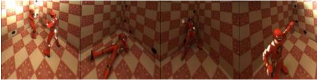
FIG. 19. An example of a polygonal panoramic image extracted from the fisheye image given in Fig. 18.
