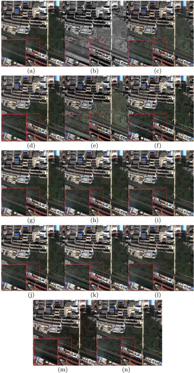
Fig. 10 Fusion results of the real QuickBird-2 dataset. a Upsampled MS image (1024×1024). b PAN image (1024×1024). c IHS method. d AIHS method. e PCA method. f BDSD method. g PRACS method. h SFIM method. i Indusion method. j MTF-GLP method. k CAE method. l MSGF method. m PNN method. n Proposed method
