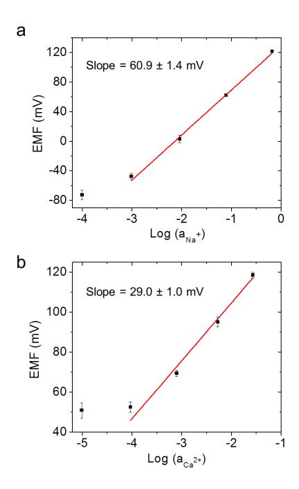
small paper- and PVC-based ISE, and a miniaturized paper-based reference electrode. Potentiometric measurements between these two electrodes make it possible to measure concentrations of electrolyte ions (Cl<sup>-</sup>, K<sup>+</sup>, Na<sup>+</sup>, and Ca<sup>2+</sup>) in aqueous solutions over ranges that are clinically useful.
