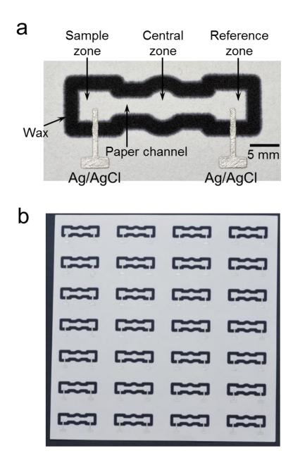
The ion-sensing EPADs are fabricated in a planar structure, and are thus appropriate for mass fabrication. As shown in Figure 1b, one page of chromatography paper (Whatman 1 Chr, 20 cm by 20 cm) can be used to fabricate 28 devices. It takes less than 30 minutes to fabricate one page of EPADs manually (28 or more devices, depending on the device configuration; *vide infra*). The efficiency of fabrication would be greatly improved by machine-based roll-to-roll printing.
