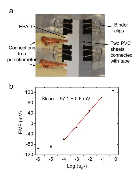
(dynamic) range of the paper devices  $(10^{-4} \text{ to } 10^{-1} \text{ M})$  is comparable to that of the conventionally assembled device (~10<sup>-5</sup> to 10<sup>-1</sup> M, Figure S5a); this observation indicates the wax-printed paper layers and the paper reference electrode function as well as the plastic/glass electrode bodies used in commercial reference electrodes.
