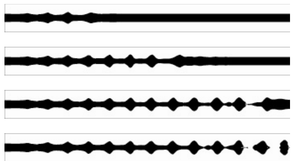
Fig. 7: Breakup of liquid jet. The inlet velocity of gas is higher than that of liquid jet. The plotted time is 20msec, 40msec, 60msec and 80msec from top to bottom.
