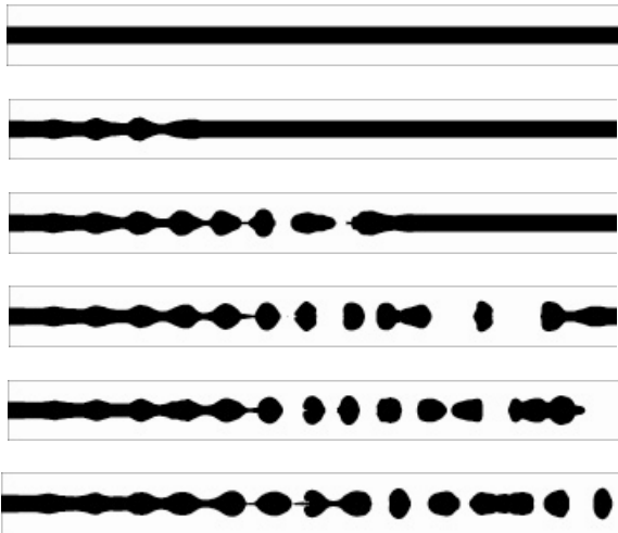
Fig. 4: Instability and breakup of liquid jet (white: gas, black: liquid). The plotted time is 0msec, 20msec, 40msec, 60msec, 80msec and 100msec from top to bottom.
