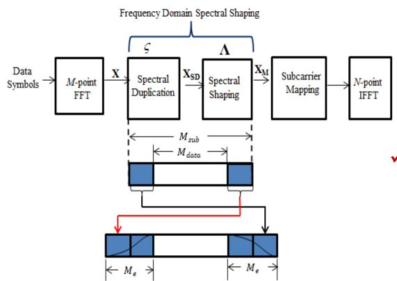
The SC-FDMA uplink requires pulse shaping to limit the inter-symbol interference (ISI) between neighboring time symbols
