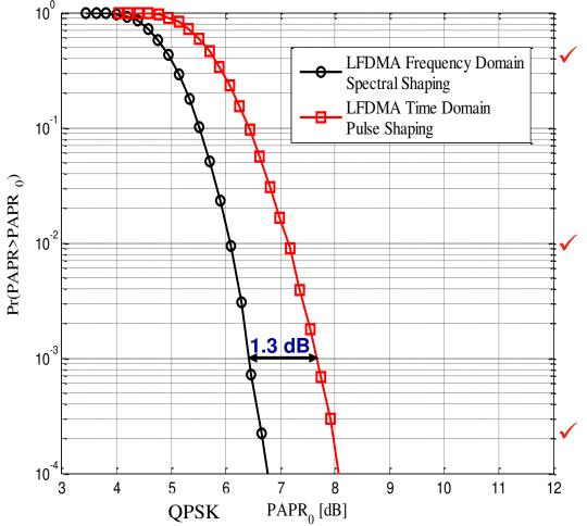
PAPR of SC-FDMA for LFDMA employed RC frequency domain spectrum shaping and time domain pulse shaping with QPSK signaling at  $\alpha$  = 0.22.
